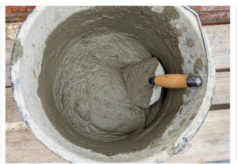
Low carbon cement: We are trialling a low carbon cement alternative, CemFree, which can save up to 80% embodied carbon compared with conventional concrete mixes. Currently, the material is in the process of becoming accredited in the UK so until then its use is limited to lightload, temporary or non-structural elements.
